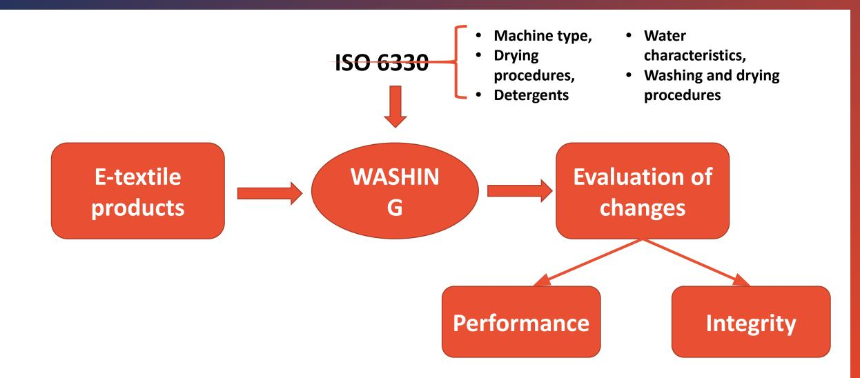
IEC 63203-204-1:2021 Wearable electronic devices and technologies - Part 204-1: Electronic textile - Test method for assessing washing durability of leisurewear and sportswear e-textile systems
