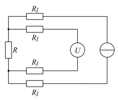
Electric diagram for the four electrode – four wire method
