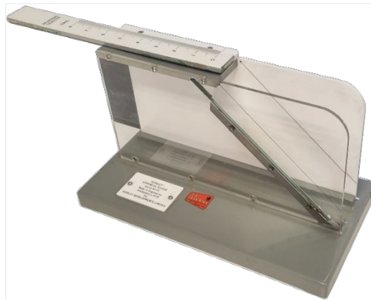
Figure 14. Equipment used to measure the stiffness.
