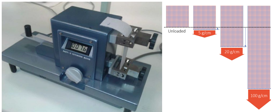
Figure 10. Picture of the instrument used to measure the extensibility (left) and loading scheme of the FAST method (right)
