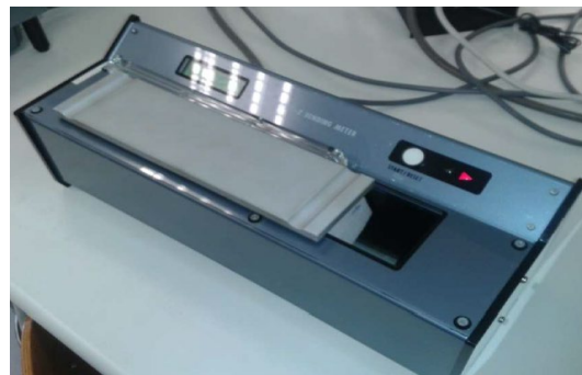
Figure 9. Image a picture of the instrument used to measure the stiffness with the FAST method
