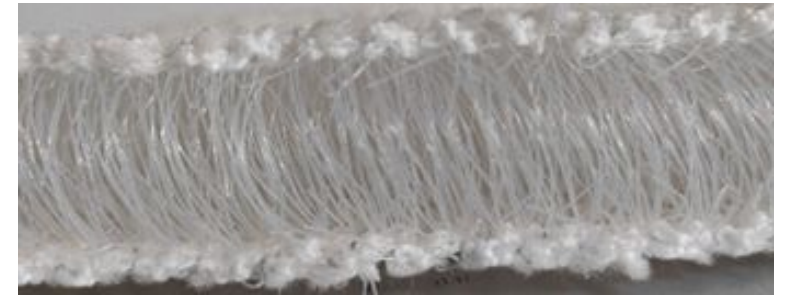
Warp knitted spacer fabric
