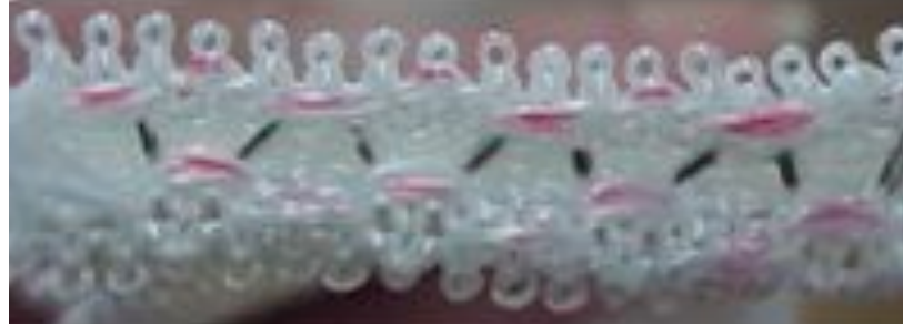
Weft knitted spacer fabric
