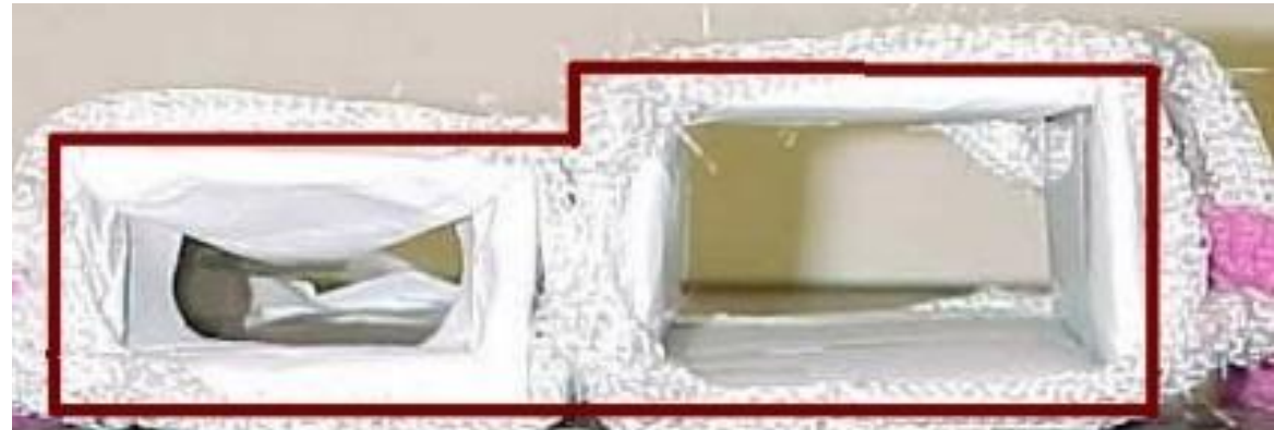
Weft spacer with connective double layers of variable length
