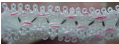
Figure 24. Aspect of a weft knitted spacer fabric, connected by yarns
