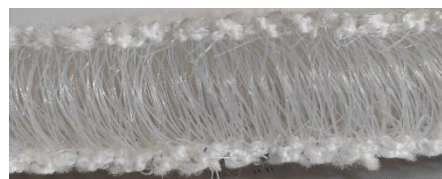
Figure 25. Aspect of a warp knitted spacer fabric
