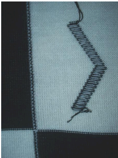
a) Example of intarsia fields with loop connection (rear aspect)
