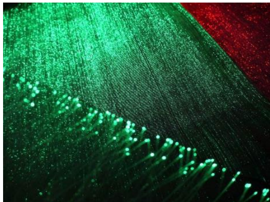
Figure 7. Light glowing fabric made with optical fibres.
