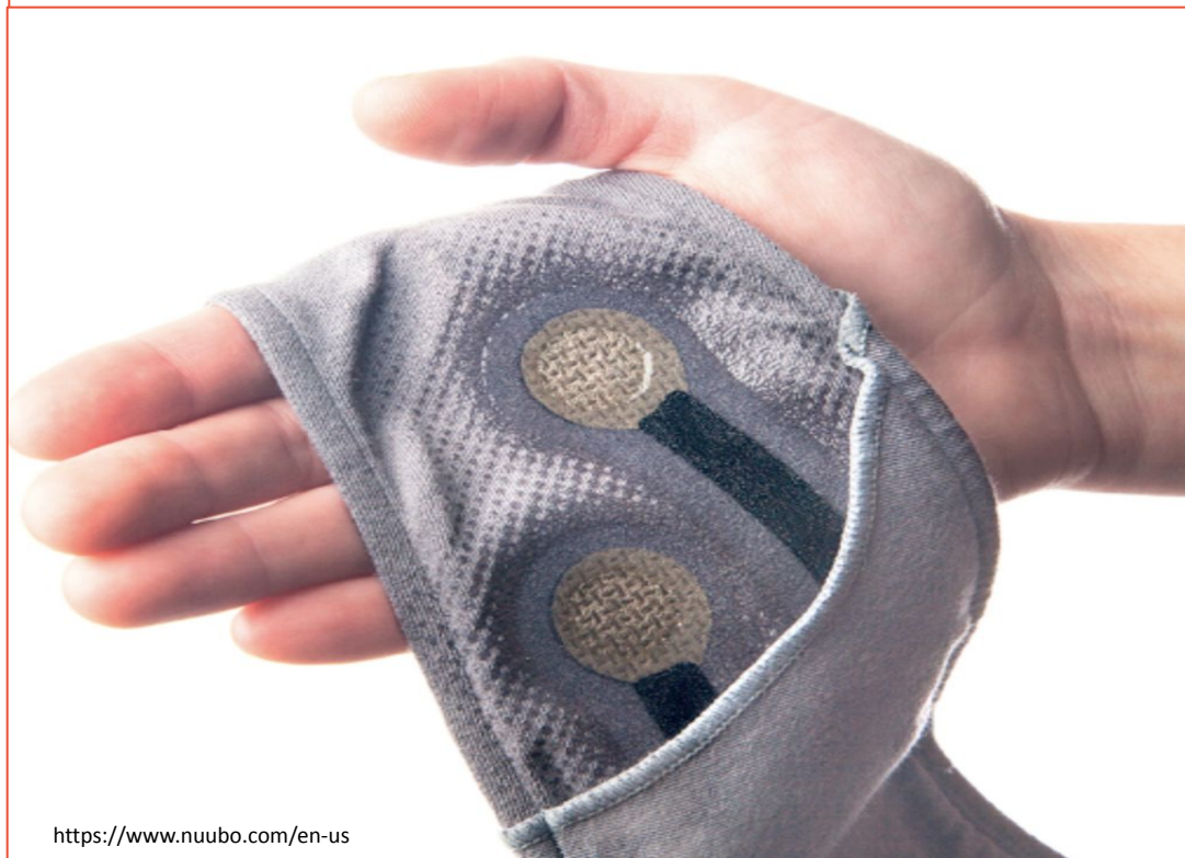
NUUBO wearable ECG unit
